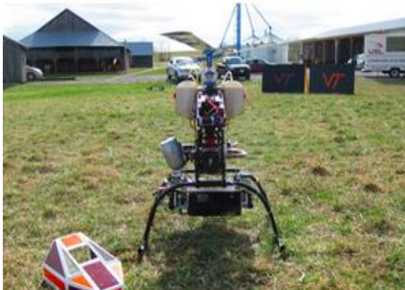
Figure 8: The helicopter with the sensor package mounted below the body of the craft.
