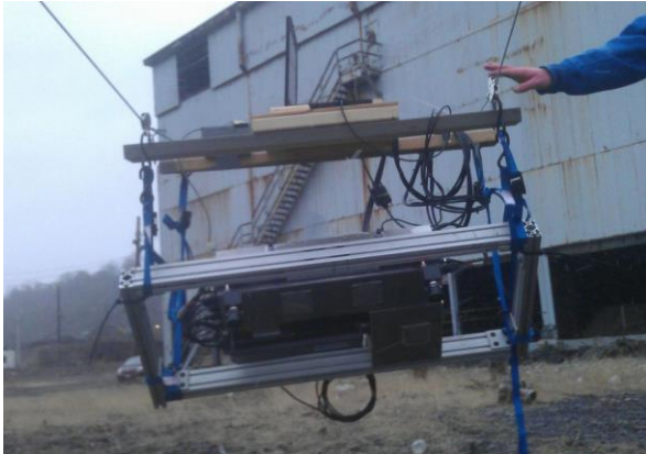
Figure 7. The zipline setup shows the sensor package hanging on cables below the computer. The cables were attached to the staircase seen in the background, approximately 10 meters off the ground.
