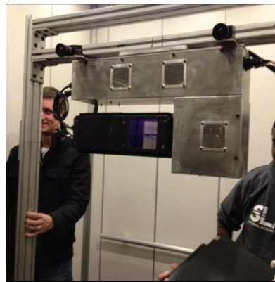
Figure 5: The sensor package, containing an IMU, stereo camera, LIDAR and microcomputer. The image shows the configuration of the sensor package mounted on the stationary frame.
