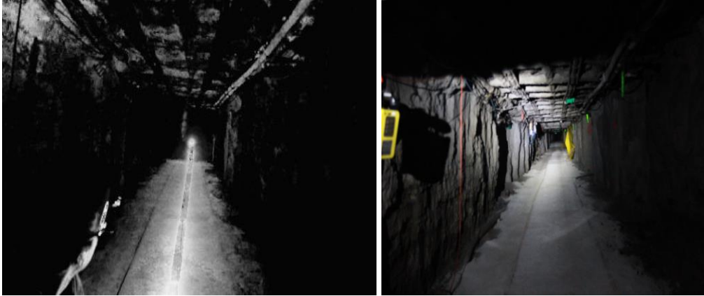
Figure 5: Image Fusion result with a sphere light made up of 18 (1 watt) LEDs (left) and Static long exposure image with 10 W head light (right) at at Bruceton Coal Mines
