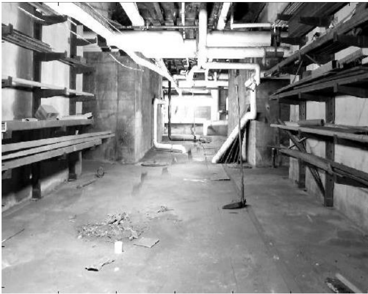
Figure 6: Image fusion result (12 ft by 6 ft by 60 ft) tunnel with 18, 1 watt LEDs arranged in a plane
