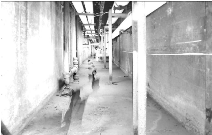
Figure 7: Image fusion result (4 ft by 6 ft by 150 ft) tunnel with 18, 1 watt LEDs arranged in a plane
